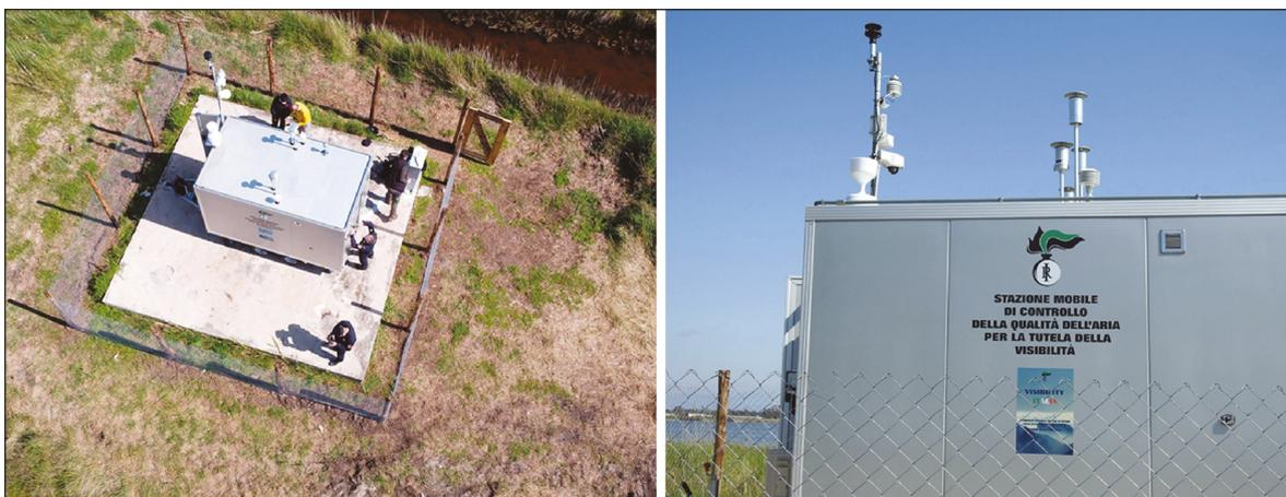
Figure 2. The Visibility cabinet near the Lago dei Monaci, drone view and focus on the sampling lines for particulate matter and the meteorological measurements.
